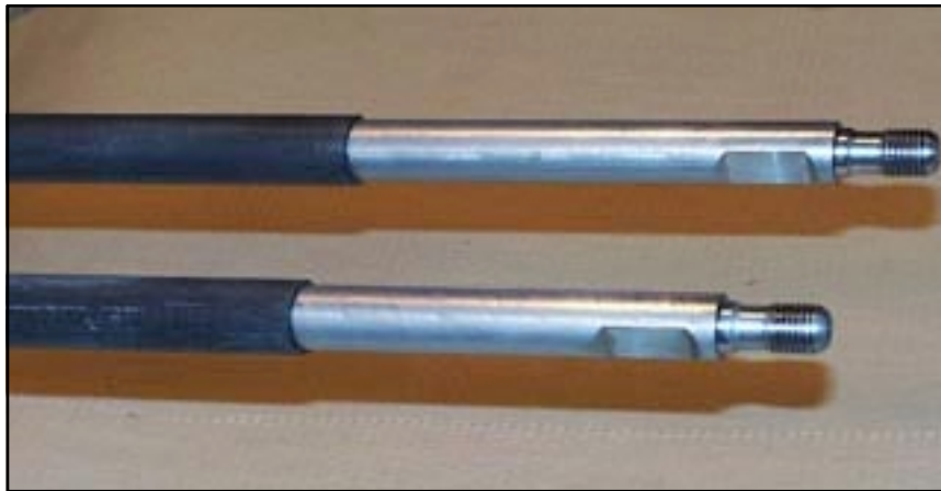
Sinkerbars sleeved with ultra high density polyethelene reduce tubing leaks even more than unsleeved sinkerbars, saving producers thousands of dollars.
